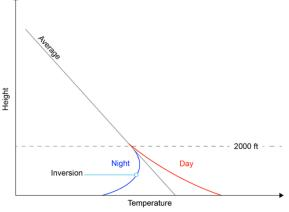
As the fog forms the lapse rate becomes approximately isothermal from the ground upwards. Loss of heat by radiation from the ground is almost completely prevented by a layer of fog
