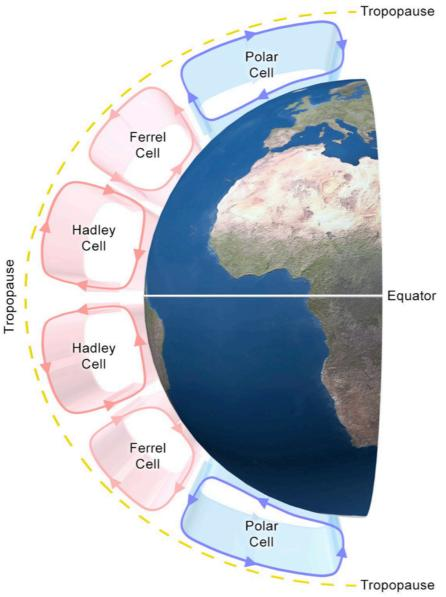
The sinking air splits at the surface, between Ferrel and Hadley, some going north and some south.
