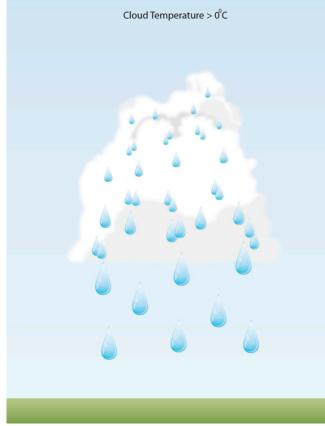
When condensation or sublimation takes place, the water droplet or ice crystal is initially about 0.02 mm in diameter with a terminal velocity of 0.012 m/s in still air
