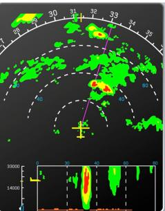
Dense clouds close to the aircraft may disguise the radar return from active cells behind it
